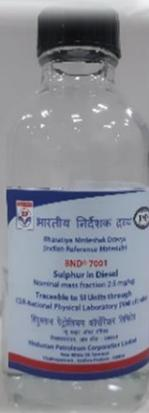
**Purpose:** Primary Standard for equipment performance check or calibration as per the standard test procedure.
