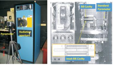
High Temperature Blackbody radiation source (MIKRON USA make Model: M390-C2) and IR-Total Radiation Pyrometer Calibration Set-up
